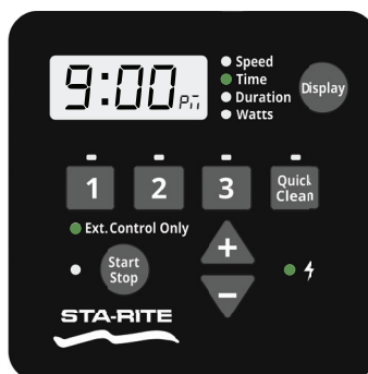
Figure 4: Activating External Control Only
